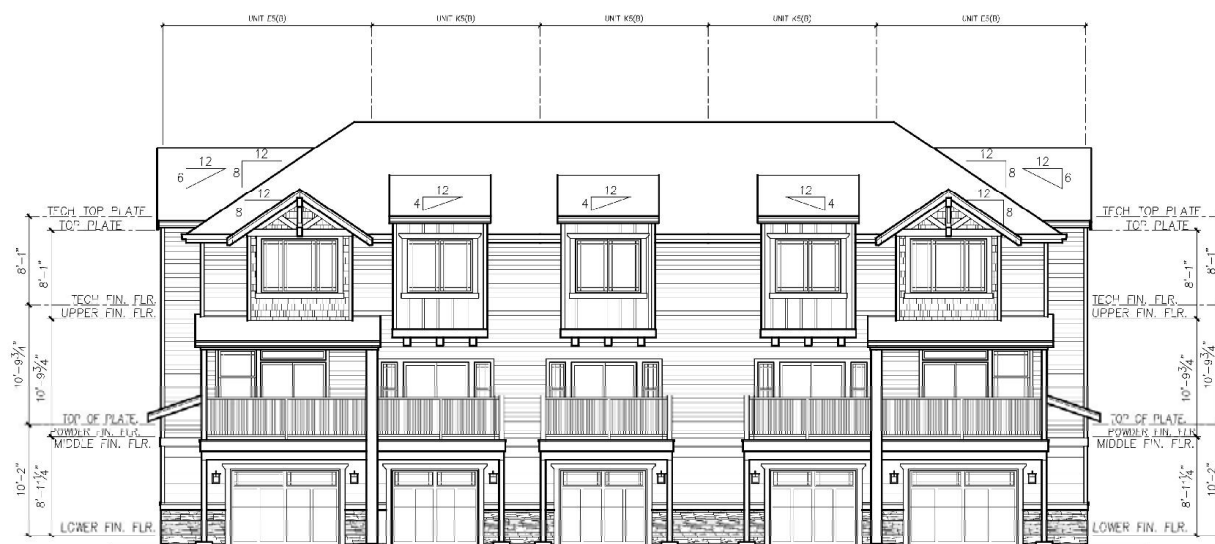
5-PLEX REAR ELEVATION 1/8" = 1'-0" AMERICAN MODERN - ALT 1
