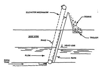
Mechanical bar screens have advantages over conventional shredders as they overcome the problem of wastewater backing up (or head loss) behind the cutters and traveling rakes bring the debris up out of the waste stream and into a solid waste container. The replacement of shredders by a mechanical bar screen at the treatment plant headworks was completed in February 1994 at a cost of \$90,399.00. (The project was originally budgeted at a cost of \$120,000.)
