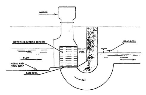
As a component of the 1981 plant expansion, the comminutor was replaced by two sewage shredders with 360 degree continuous cutting capability. The shredders normally operated without interruption unless jammed by a bolt, rock or similar object. When this should happen, the shredder's control panel automatically reverses cutter rotation to dislodge the object.
